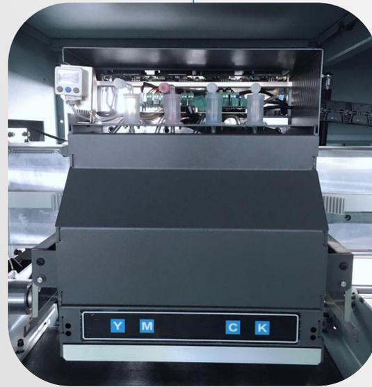
Large-capacity color separation circulation ink cartridges, ensures long time printing without any ink break
