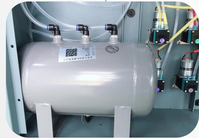
Double large-capacity negative pressure gas tank, enhances the buffer time of pressure, make ink circulation more stable & fluency.
